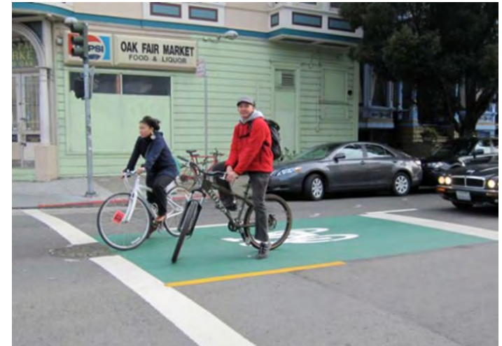
Example bicycle box Source: Inhabit.com
