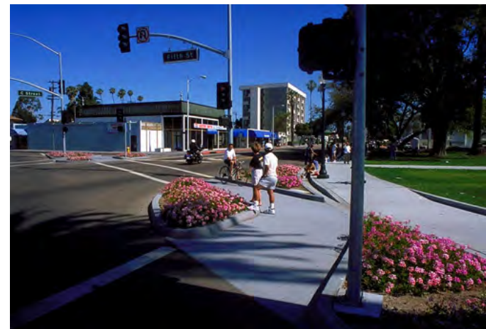
Example curb extensions Source: pedbikeimages.org
