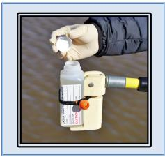
Fill the Ammonia sample bottle to the fill line, and immediately replace the cap. If there is no clear fill line, fill it to the "neck" of the bottle.
