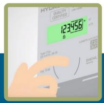
Find the "meter read" and "flow rate" screens. The "meter read" is above.
